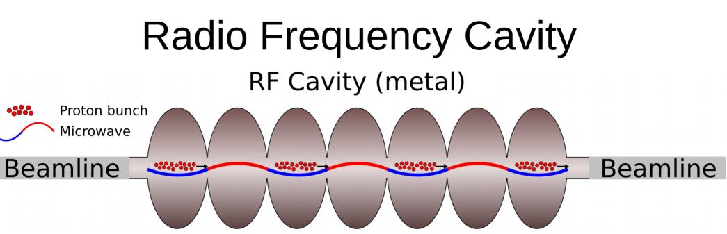
Metal amplifies the microwave Very high wattage, driven by klystron machine
